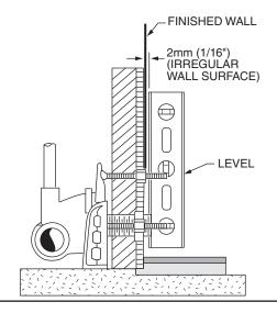
■ NOTE: Bearing nuts and washers must be set to take full loading from the fixture allowing 1/16" (2mm) clearance between fixture and wall.
