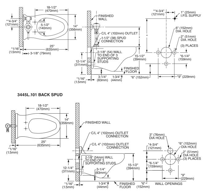
\* THESE DIMENSIONS MUST BE MAINTAINED FOR PROPER INSTALLATION \*\*VARIABLE-CHECK WITH MANUFACTURER OF FLUSH VALVE FOR PROPER ROUGH-IN
