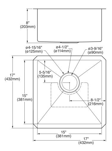
**NOTES:** \* DIMENSIONS SHOWN FOR LOCATION OF SUPPLIED AND "P" TRAP ARE SUGGESTED. FITTINGS NOT INCLUDED WITH FIXTURE AND MUST BE ORDERED SEPARATELY. SEALING COMPOUND SUPPLIED BY OTHERS.
