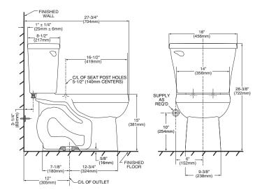
THIS COMBINATION IS DESIGNED TO ROUGH-IN AT A MINIMUM DIMENSION OF 305MM (12") FROM FINISHED WALL TO C/L OF OUTLET.
