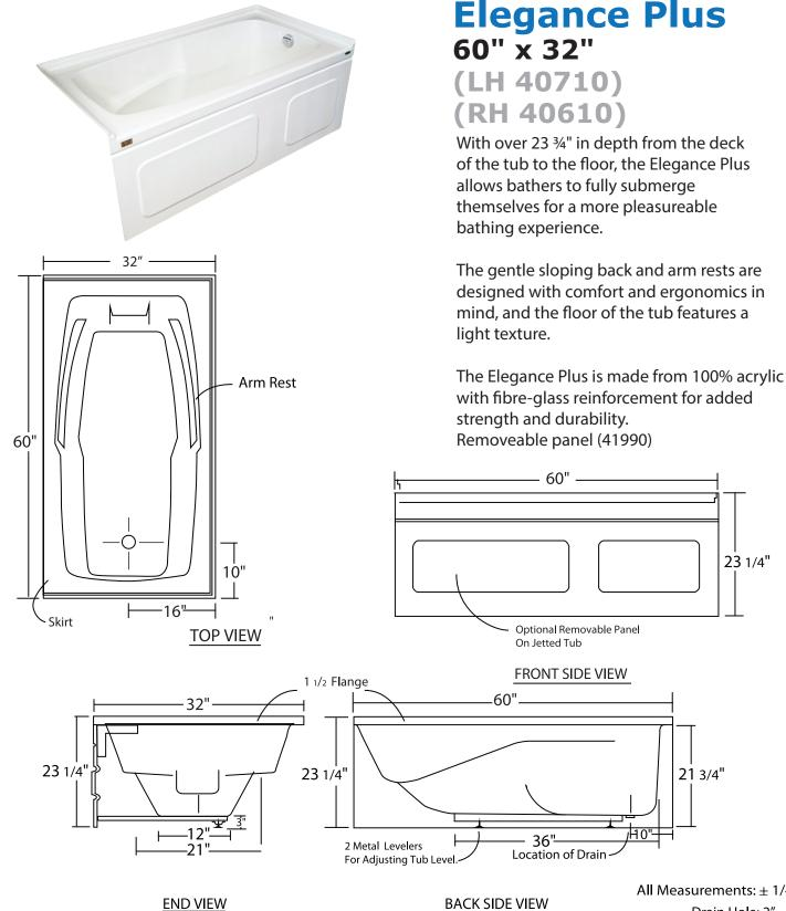
All Measurements: ± 1/4" Drain Hole: 2" Overflow Hole: 2 1/2"
