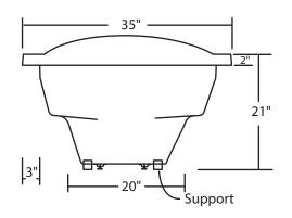
Drain Hole: 2" Overflow: 2 1/4" Sizes: <u>+</u> 1/4"
