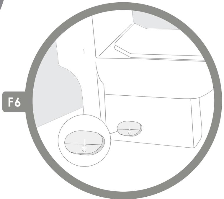
**10** Turn on supply valve and allow tank to fill until float rises to shutoff position. Then place the tank lid on top of the tank.
