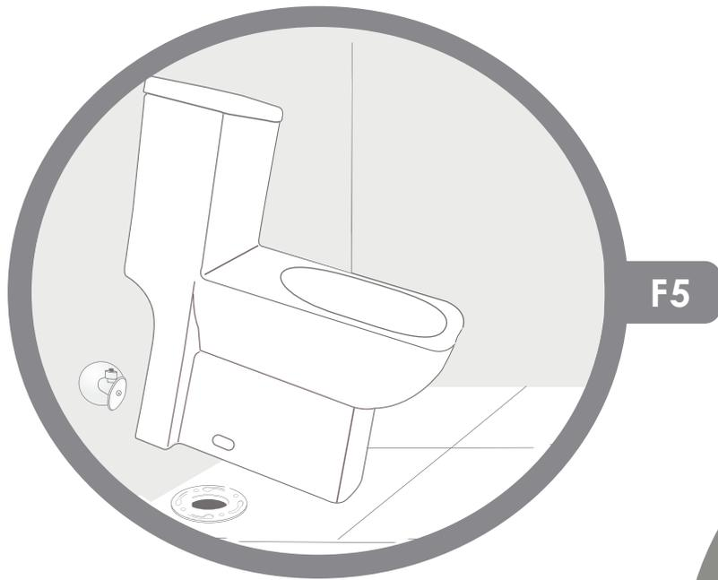
**06** Lower the toilet onto the floor bolts, so the floor bolts project through the mounting holes in the base of the toilet (F5). Using a rocking motion, press the bowl down to position the toilet onto the flange and create a seal with the wax ring.
