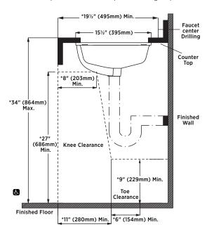
Note: \* Starred measurements comply with ADA and OBC barrier free accessibility requirements.
