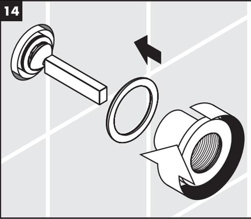
Install the washer and sleeve/escutcheon assembly.
