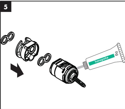
Install the cartridge adapter and sealing rings on the cartridge.
