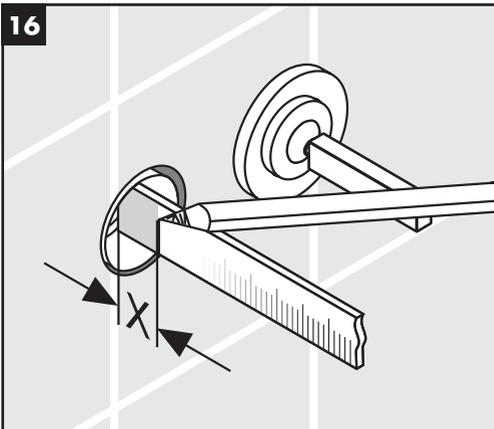
Measure the distance from the surface of the spout port rough to the outside edge of the plaster shield ("X").
