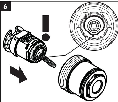
Insert the cartridge in the cartridge cover, oriented as shown on the diagram.
