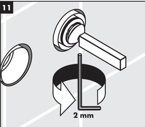
Tighten the handle screw using a 2 mm Allen wrench.
