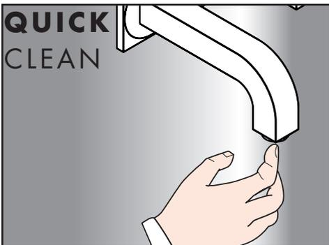
The aerator uses QuickClean cleaning system. Deposits of mineral scale can be removed by rubbing across the channels with a finger or sponge.
