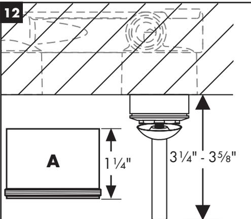
Measure the distance between the wall and the edge of the handle.
