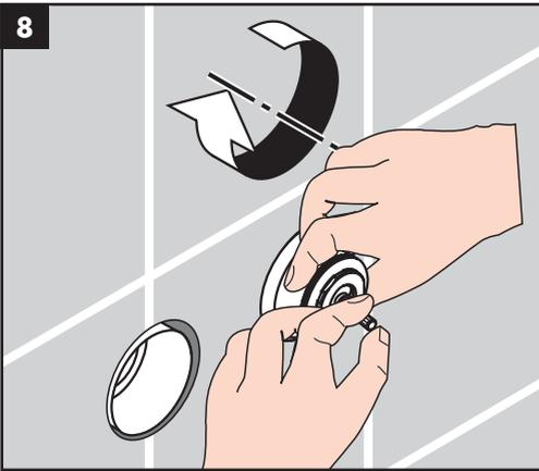
Hold the cartridge stem steady with one hand.
