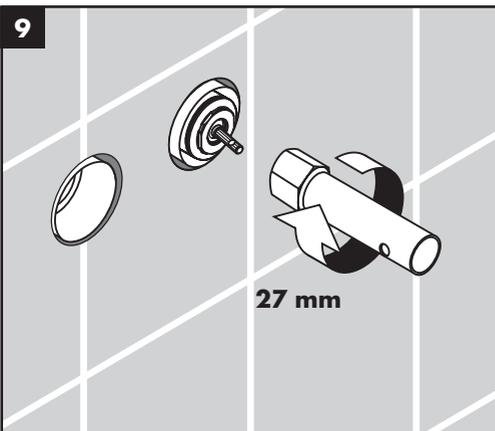
Tighten the cover using a 27 mm wrench.
