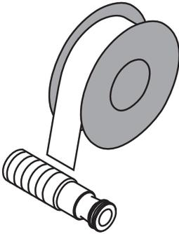
Wrap the threads on the nipple with Teflon tape.
