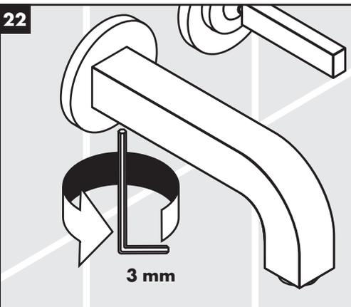
Tighten the spout screw using a 3 mm Allen wrench.
