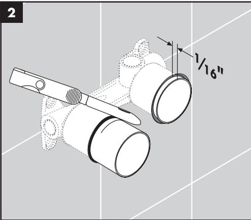
Cut the plaster shields so that they extend  $\frac{1}{16}$ " outside the surface of the finished wall.
