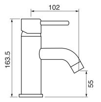
Includes push drain 3/8" flexible supply hose 1.5 GPM (5.7 L/min.)
