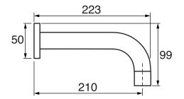
25mm diameter spout 1/2" male NPT inlet Sliding flange
