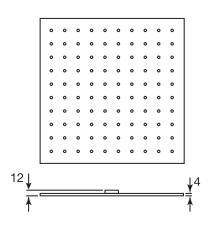
4 mm in thickness Easy clean nozzles High polished stainless steel 2.5 GPM (9.5 L/min.)
