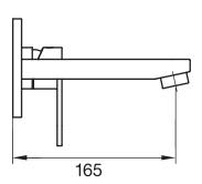
Lead free brass Drain not included 3/8" flexible supply hoses 2 GPM (7.5 L/min.)
