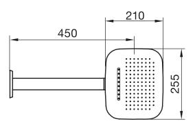
Wall arm included 2 function rain shower with rain stream Easy clean nozzles 2 GPM (7.5 L/min.)
