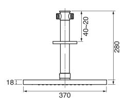
Ceiling arm included 2 function rain shower with rain stream Easy clean nozzles 2 GPM (7.5 L/min.)
