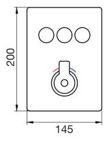
Thermostatic valve with PushGo technology – 3 controls Multiple outlets can be run simultaneously Includes rough-in Instant flow when on 5 GPM (18.9 L/min.)
