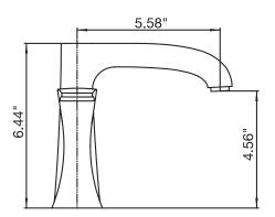
Includes push drain 1.5 GPM (5.7 L/min.)
