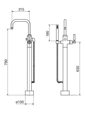
Includes rough-in 5 GPM (18.9 L/min.)
