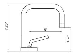
Includes push drain 3/8" flexible supply hoses 1.5 GPM (5.7 L/min.)
