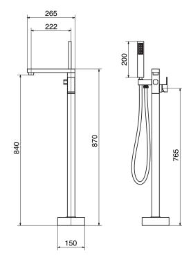
Includes rough-in 5 GPM (18.9 L/min.)
