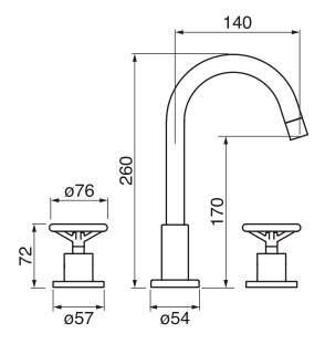
Includes push drain 1.5 GPM (5.7 L/min.)
