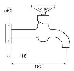
Drain not included 1.5 GPM (5.7 L/min.)
