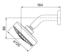
Large diameter face – 4<sup>3/4</sup>" 3 position spray with massage Easy clean nozzles 2.2 GPM (8.3 L/min.)
