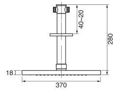
Ceiling arm included 2 function rain shower with rain stream Easy clean nozzles 2 GPM (7.5 L/min.)
