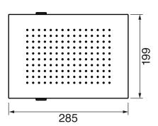
Stainless steel construction Easy clip installation 1/2" NPT male connection 2.5 GPM (9.5 L/min.)
