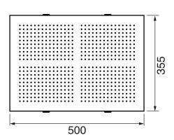
Stainless steel construction Easy clip installation 1/2" NPT male connection 2.5 GPM (9.5 L/min.)
