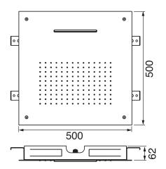
20" x 20" (500 mm x 500 mm) Easy clean nozzles Recessed built in frame High polished stainless steel Rain – 2.5 GPM (9.5 L/min.)
