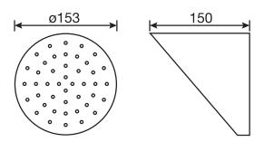
Easy clean nozzles High polished stainless steel Includes mounting bracket 2.5 GPM (9.5 L/min.)
