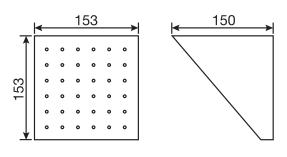
Easy clean nozzles High polished stainless steel Includes mounting bracket 2.5 GPM (9.5 L/min.)
