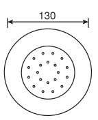
Directional head Easy clean nozzles 1.5 GPM (5.7 L/min.)
