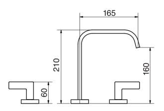
Includes push drain 1.5 GPM (5.7 L/min.)
