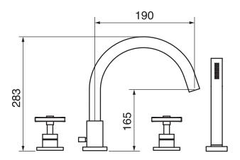
8 GPM (30.3 L/min.)
