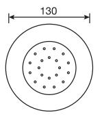
Directional head Easy clean nozzles 1.5 GPM (5.7 L/min.)
