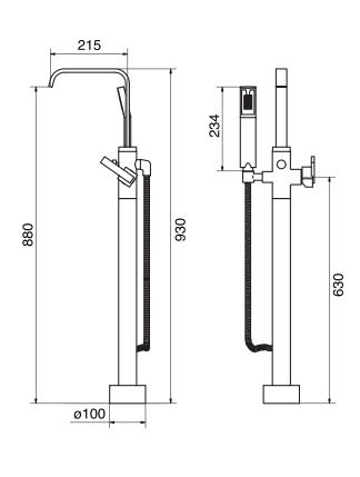
Includes rough-in 5 GPM (18.9 L/min.)
