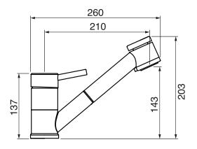
Pull out hand shower with dual function spray Swivel spout 2 GPM (7.6 L/min.)
