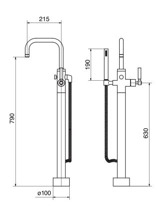
Includes rough-in 5 GPM (18.9 L/min.)
