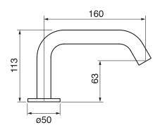
Includes push drain 1.5 GPM (5.7 L/min.)
