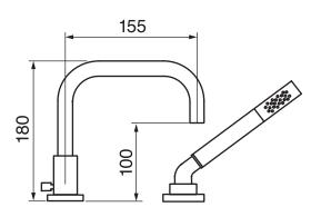
8 GPM (30.3 L/min.)
