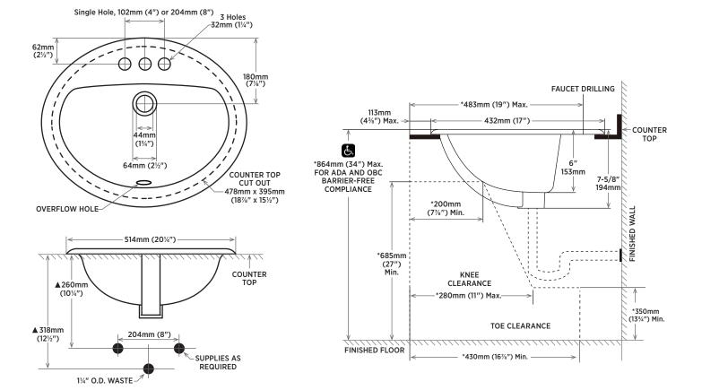
NOTE: \* Starred measurements comply with ADA and OBC barrier free accessibility requirements. A Dimensions shown for location of supplied and waste are suggested.
