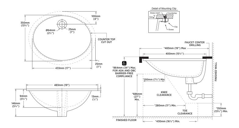
NOTE: \* Starred measurements comply with ADA and OBC barrier free accessibility requirements.
