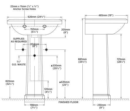
NOTE: ▲ Dimensions shown for location of supplied and waste are suggested. Actual dimensions must be taken from fixture.
