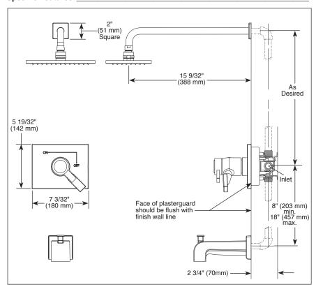
**RP62955**▲ (2.5 GPM) **RP91363**▲ (1.75 GPM) Touch-Clean<sup>®</sup> Raincan
