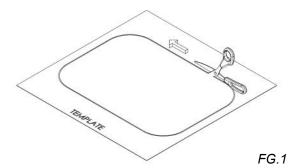
1. Using the template provided, mark the shape to be cut out on the counter. FG.1
