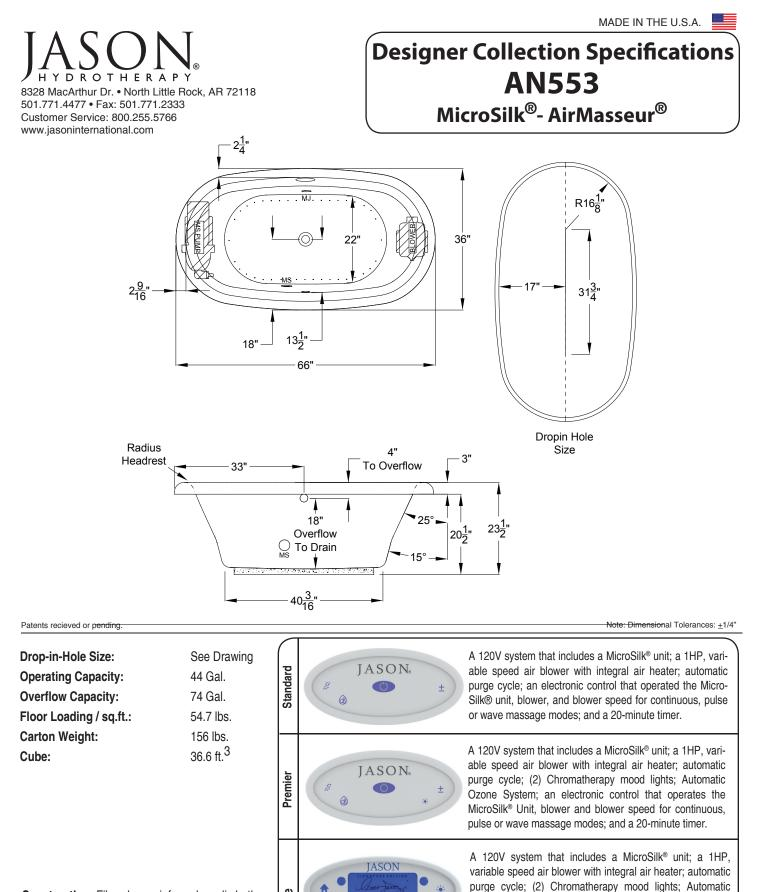
**Construction:** Fiberglass reinforced acrylic bath with Level Form<sup>™</sup> full-support base.
