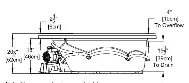
Note: The pump extends approximately 1" past the end radius of the bath. This requires angling the bath into the drop-in hole.
