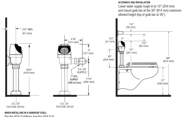
Per the ADA Guildlines (section 604.9.4) it is recommended that the grab bars be split or shifted to the wide side of the stall. If grab bars must be present over the valve, use the alternate ADA installation as shown to the right.
