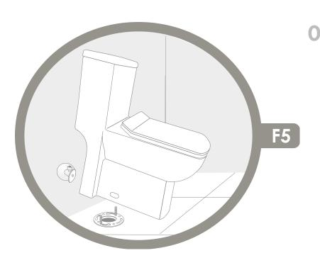
Lower the toilet onto the floor bolts, so the floor bolts project through the mounting holes in the base of the toilet. (F5) Using a rocking motion, press the bowl down to position the toilet onto the flange and create a seal with the wax ring.
