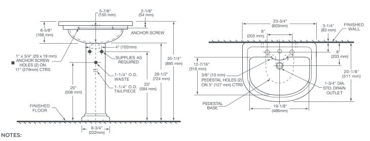
Dimensions shown for location supplies and "P" trap are suggested. Provide suitable reinforcement for all wall supports. Slab/pedestal anchors and mounting features to be furnished by others.
